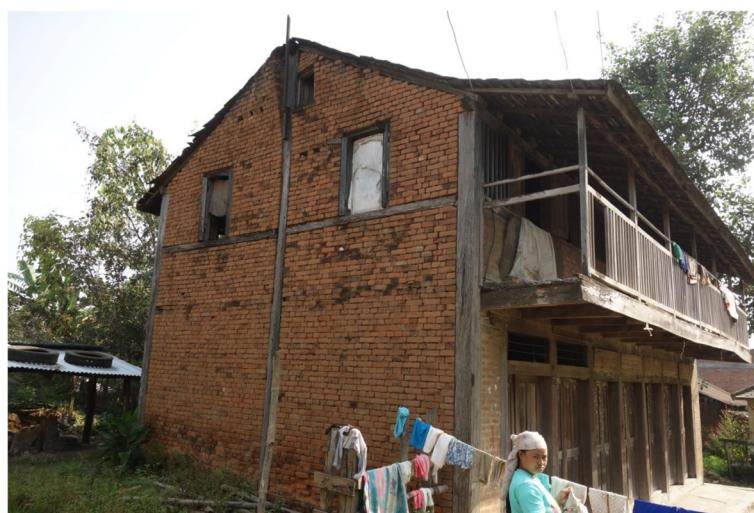
**Fig. 14** A house with timber lacing and corner posts in the same stretch of western Nepal which survived during 1988 and 2015 earthquakes
