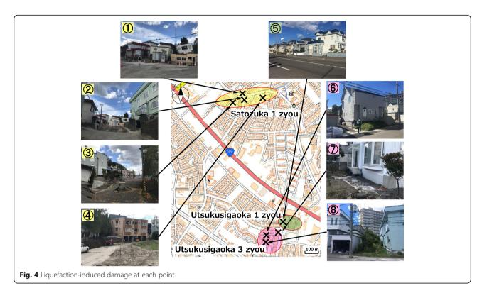
4-① to ③. In this area, tension cracking was not seen so much, so it can be inferred that the lateral spreading is not large.
