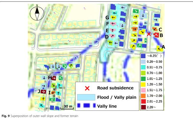
Utsukushigaoka in Sapporo city are focused. The damage at Satozuka was so serious that the residents could not continue to live there. Although the inclination of houses can be seen by visual inspection at Satozuka, there were few houses where the inclination can be judged visually at Utsukushigaoka. Terefore we did a field survey of inclined houses by using a digital angle meter in Utsukushigaoka.
