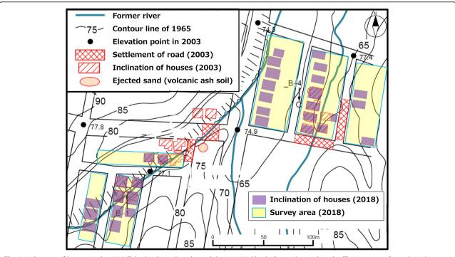
Fig. 7 Inclination of houses in the 2003 Tokachi-oki earthquake and the 2018 Hokkaido Iburi-tobu earthquake (The Japanese Geotechnical Society 2018)
