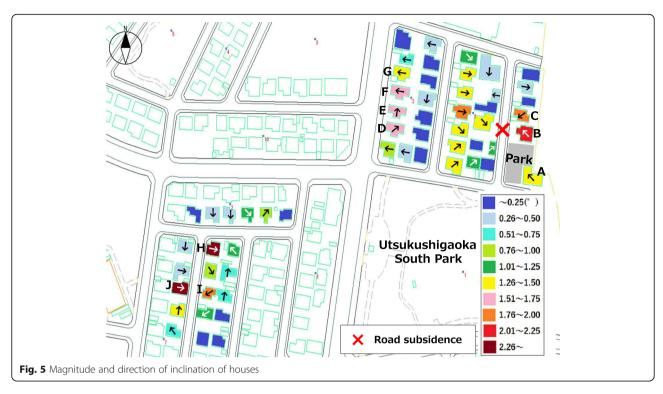
such houses are inclined in the same direction according to Fig. 5. The houses were also inclined in the direction of the largest subsided road. These houses have almost the same wooden structure and were constructed 29 years ago.
