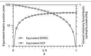
**Fig. 8** Equivalent matric suction and hydraulic conductivity function against degree of saturation of the model
