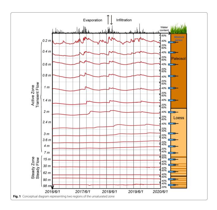
season, and water content remained basically unchanged at a depth exceeding 1 m (Russo and Fiori 2008). The upper wetting zone is commonly referred to as the "active zone", whereas the underlying zone with an unchanged water content is referred to as the "steady zone". Past scientific understanding had been that piston flow occurred in the active zone, whereas there was no flow in the steady zone (Gazis and Feng 2004).
