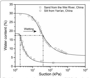
**Fig. 6** Representative soil water retention curves (SWRC) of sand and silt from China
