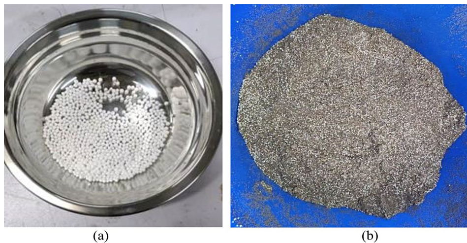
Fig. 2 Buffering materials: (a) EPS beads; (b) EPS bead-sand mixture
