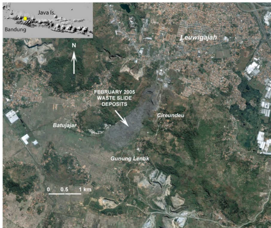
Figure 1 Location of the 21 February 2005 waste avalanche at Leuwigajah, Bandung, in Java Island. High-resolution satellite image as of 3 August 2006 (source: GoogleEarth).
