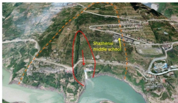
Fig. 4 Alert zones defined in the emergency response. The red lines delineate the actual extent of the landslide range, and the dotted orange lines delineate the alert zones before the collapse. No residents live on the opposite bank of the Luogudong River, and that hence that area is excluded from the alert zone
